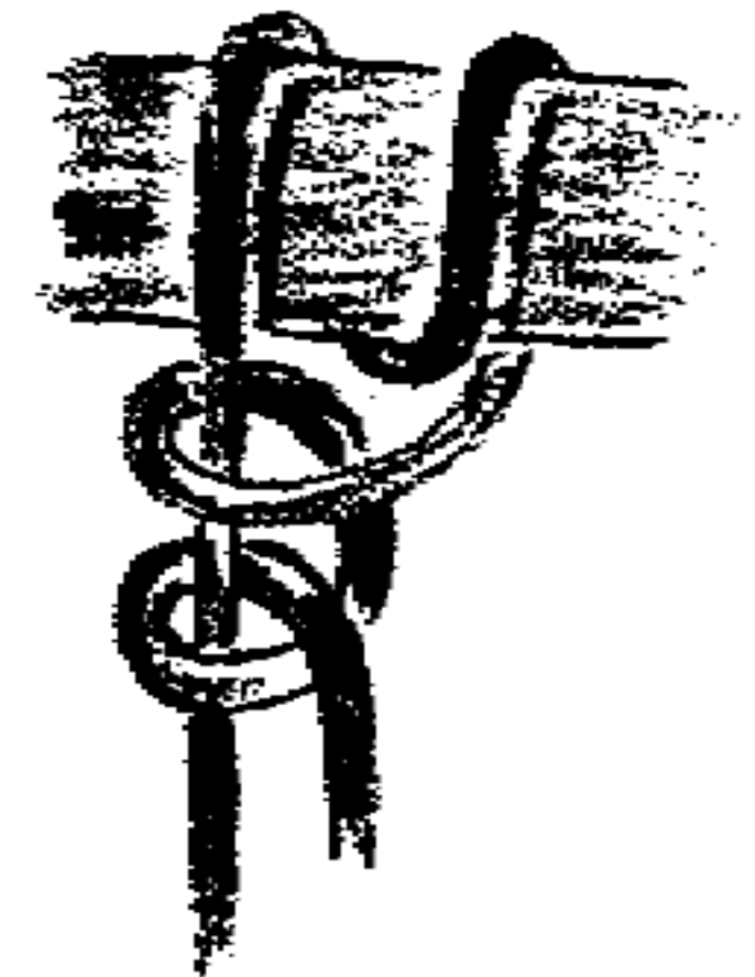
k Round Turn—Two Half Hitches. Mooring knot.
