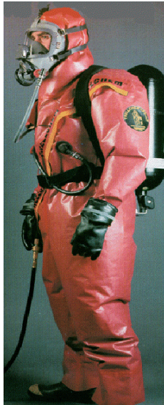
Figure B-2. Level B Protection
