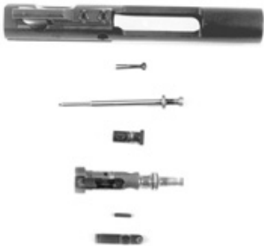
Figure 2-17. Bolt Carrier Disassembled.
