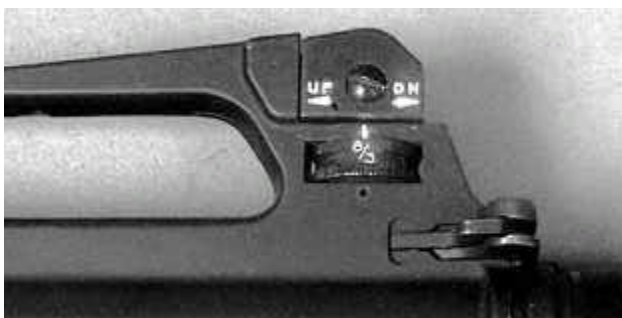
Figure 9-6. Rear Sight Elevation Knob Set for 300 Yards/Meters.
