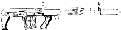
Preproduction models with different butts and pistol grips. The foregrip differs from the production model.
