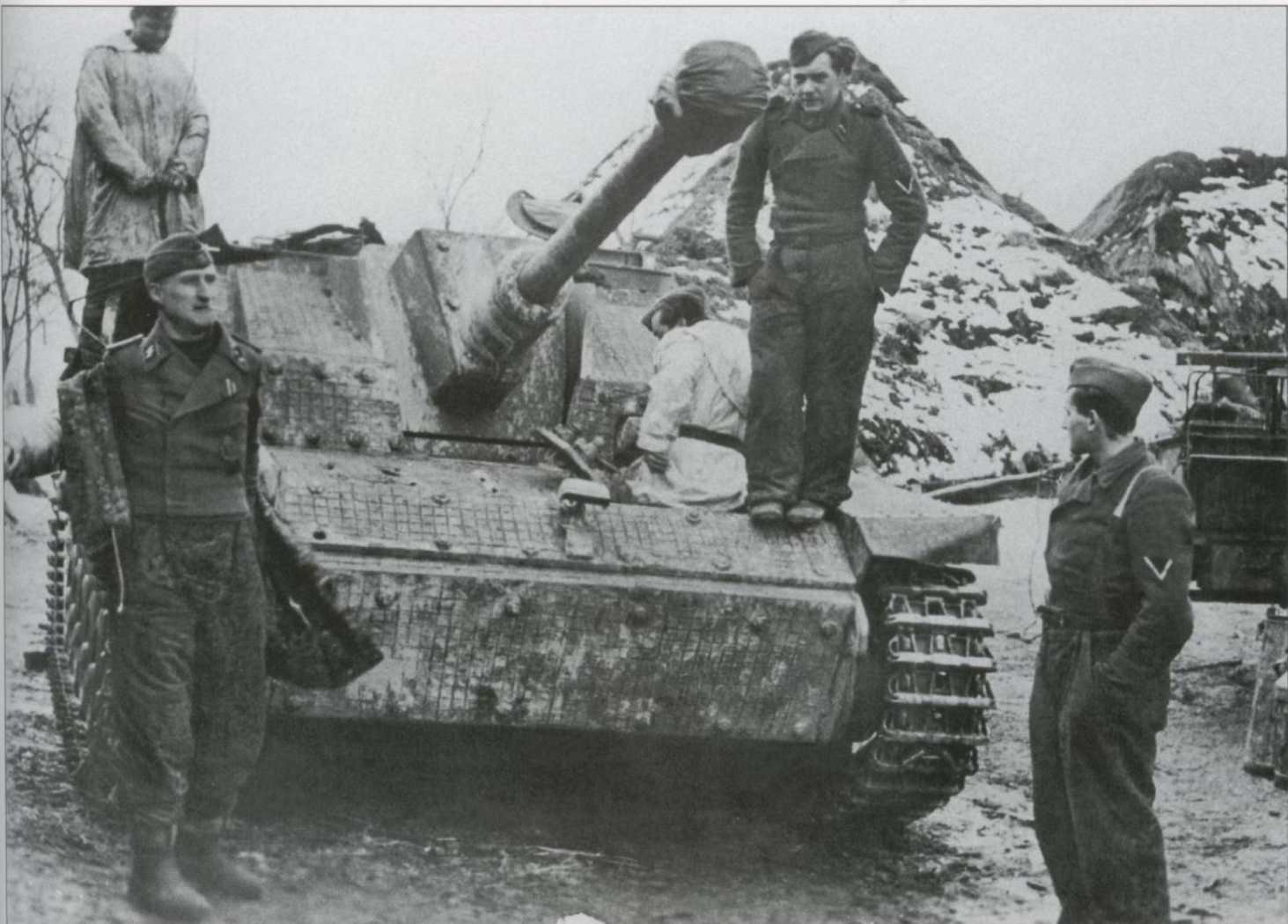
Here a StuG crew prepares to go into action. The commander at left is putting on a reversible winter uniform, with the autumn side in, over the standard gray jacket worn by armored troops. The checkered texture on the armor of the assault gun is Zimmerit , a paste that was applied to protect the armored vehicle against antitank mines.
