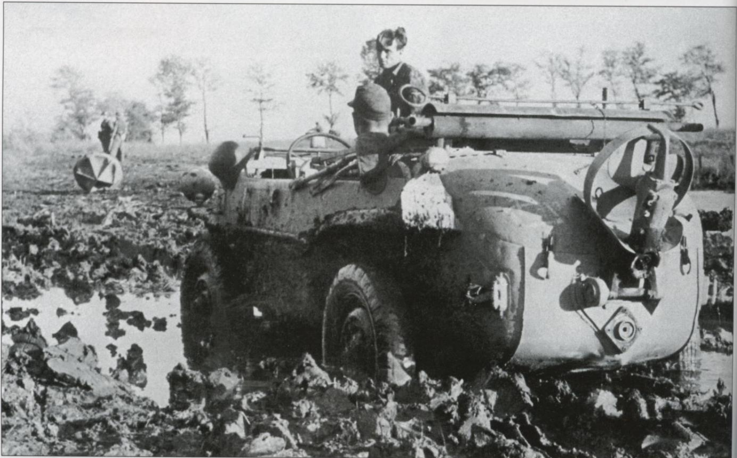
An SS Schwimmwagen slowly advances through the mire in a muddy stretch of land in Russia. If the terrain were any wetter, the driver would be compelled to lower the propeller at the rear of the vehicle to boost his speed. Note the markings that are visible just to the left of the propeller.
