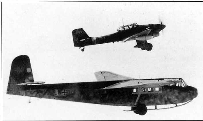
No uncertainty about this Ju 87R, however. The DFS 230 glider in the foreground and the tow-hook attachment behind the tailwheel clearly identify it as a glider-tug of II./LLG 1
