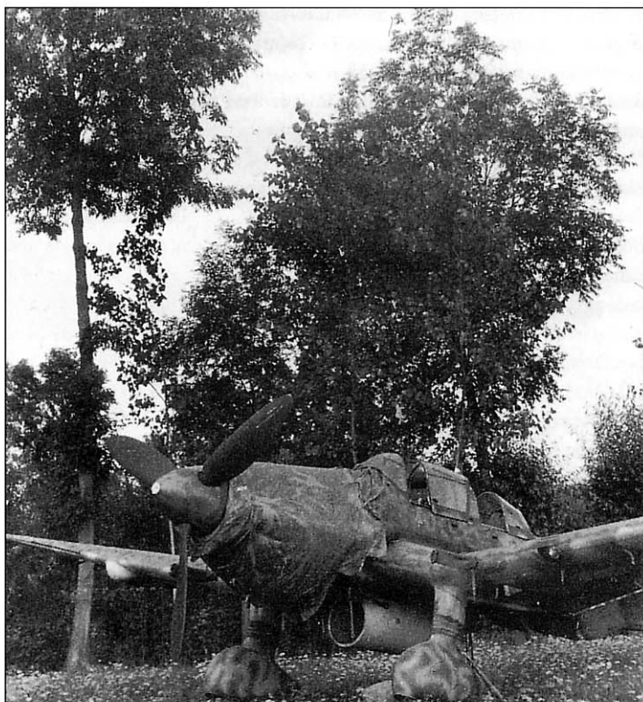
Another NSGr 9 Dora in a similar finish awaits the coming night's operations dispersed among the trees bordering an unidentified Italian airfield. Note the tarpaulin covering the engine, and the Universal-Behälter , or GP stores container – minus its nose cap – attached to the ventral bomb fork
