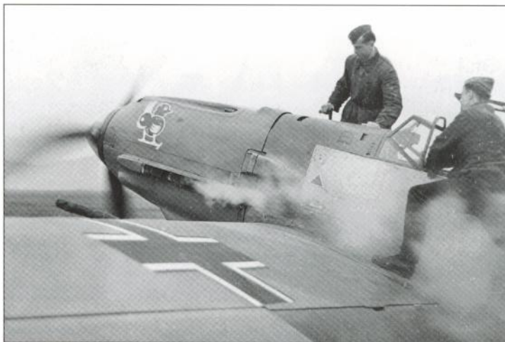
Offering a good close-up of 8./JG 54's 'Piepmatz' emblem, this photograph shows the DB 601 engine of a yellow-cowlinged Bf 109 coughing protestingly into life as the mechanic on the wingroot reaches into the cockpit to ease back the throttle. The 'black man' on the far side, his work done, removes the starter handle
