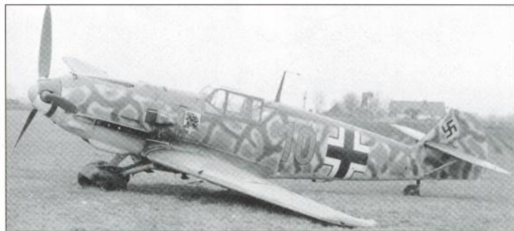
. . . and 'Yellow 10', an E-4/B (note ventral bomb rack), whose new paintwork cannot disguise an old problem – the inherent weakness of the Bf 109's spindly undercarriage
