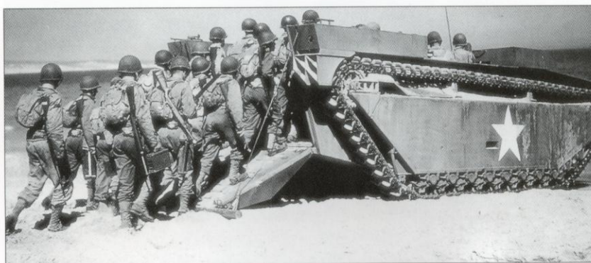
Loading an amtrac; the LVT-4 of 1944 could hold about 34 passengers, and had a rear ramp, which made loading and unloading much easier and safer. Note the gull-winged track pattern. These men all carry the M1936 musette as a pack.
