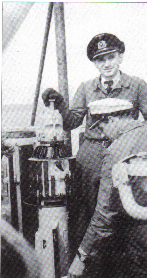
One of the most important pieces of equipment on the bridge of a U-boat was the Überwasserzieloptik , generally referred to as the UZO . A pair of special binoculars was attached to the top of this pedestal device and used to transmit target settings for the torpedoes. The IWO , Oberleutnant Pietschmann , rests his gloved hand on the UZO on the bridge of U-377, a Type VIIC. (Jak P. Mallmann-Showell)
