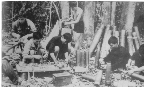
A VC jungle workshop manufacturing large explosive booby traps from salvaged US munitions components. Two men to the left prepare detonators and fuses. To the right are 105mm projectiles that will be used for booby traps. The 105mm brass cases and the steel propellant and fiber projectile containers behind them will be made into "pipe bombs."
