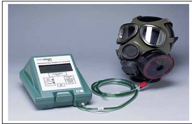
Figure A-6. M41 Protection Assessment Test System
