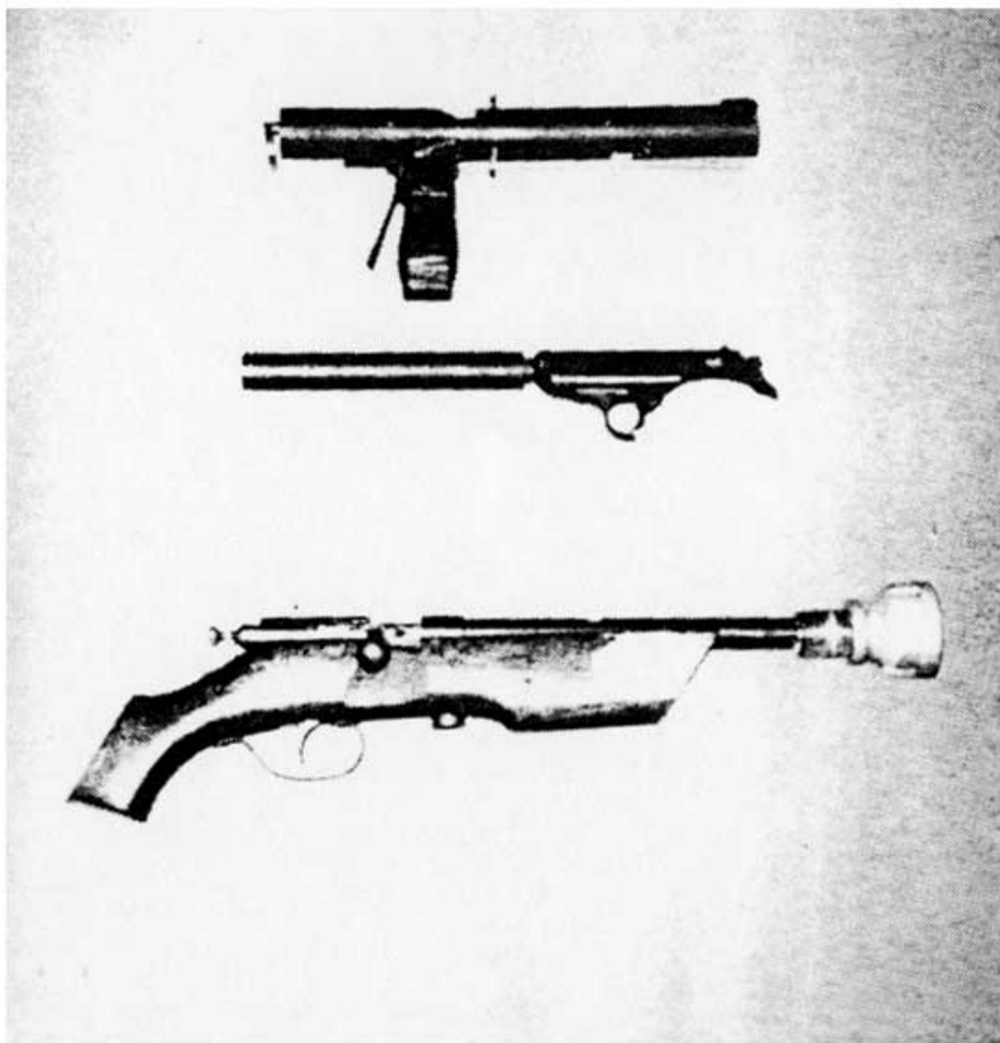
SILENT PISTOLS Top to bottom i Librod 22 cal ii PPK .22 cal with Parker-Hale moderator iii Cut-down .22 rifle with bell reducer (point blank) silencer-muzzle to skin
