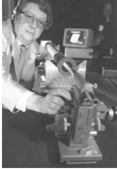
Left: This is a multilayer water-window imaging X-ray microscope being demonstrated by its inventor. Right: A basic schematic of the main parts of an X-ray microscope. This illustration is from the Lawrence Livermore National Labs Web site on high-energy lasers recommended in the Resources section. [NASA/Marshall news photo, 1992; LLNL tutorial photo, released.]
