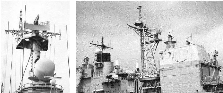
Left: A variety of types of radar antennas are visible on the Soviet-built USNS Hiddensee, including a High Pole-B EW antenna, a Square Head Identification Friend or Foe (IFF) receiver on the back, a Plank Shave missile-targeting antenna on the front, a Kivach 3 surface-search antenna on the bridge, and a radome with a Bass Tilt gunfire control antenna to control two types of gun systems. Right: The U.S. Navy cruiser USS Normandy (CG-60) is equipped with a cone-shaped SPQ-9A surface gun control radar on the fore mast, an SPG-62 radar illuminator to the left, an SPS-29(V)6 air-security radar on the main mast with a small dome-shaped SPS-64(V)9 navigational radar above and forward on the mast. On the top aft deck are two SPG-62 radar illuminators and on the right is a QE-82 antenna for WSC-3 UHF Satcomm. On the aft deck house are two panels of the SPY-1A fixed antenna radar array. [U.S. DoD 1993 and 1994 news photos by Don S. Montgomery, released.]
