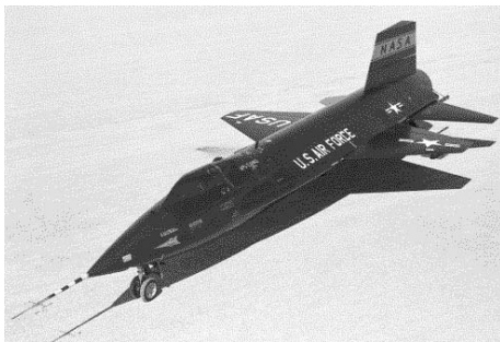
The X-15 was a rocket-powered, missile-shaped aircraft designed for high-altitude testing and the deployment of scientific sensing and data-collection instruments. Like the later Space Shuttle, the X-15 was launched from another craft at high altitude, in this case a B-52 aircraft (right). It would then glide in powerless flight and execute a glide landing. There is an X-15 rocket plane exhibited in the National Air and Space Museum in Washington, D. C. [NASA/ Dryden Flight Research Center 1960 and 1968 news photos, released.]
