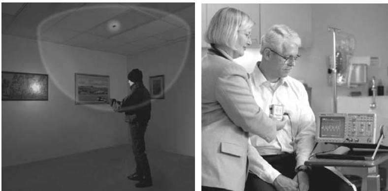
Left: A concealable radar security detector can sense intruders up to a distance of six meters. Designed at the Lawrence Livermore National Laboratory (LLNL), the repeat radar signal from this micropower impulse radar (MIR) detects motion in the room by responding to changes in the returning echo. Right: The same impulse radar technology can be used to peer into novel places, as shown with this micropulse radar stethoscope used by Elaine Ashby, M.D., to measure inventor Tom McEwan's heart rate. [LLNL news photos by Jacqueline McBride and James E. Stoots, Jr., released]
