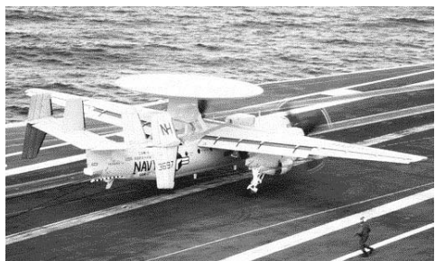
Left: A Joint Service team assembles an Army-Navy Transportable Ground 75-Air Control and Warning Radar System on the McGregor Test Range in New Mexico. Right: An Airborne Early Warning E-2C Hawkeye lands on an aircraft carrier. Note the streamlined radar-protecting radome on top of the craft. [U.S. DoD 1996 news photo by Regina Height and 1990 news photo by Don S. Montgomery, released.]
