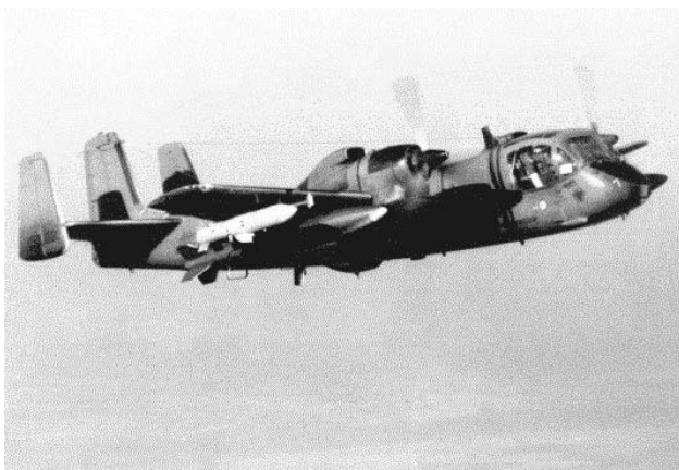
This is a Grumman OV-1C aircraft, called the Mohawk, which came into production in 1959 as a reconnaissance and photo-observation craft for the U.S. Marines and the U.S. Army. The "C" designation indicates that the aircraft was equipped with an infrared electronic reconnaissance imaging system. [NASA/Dryden Flight Research Center 1983 news photo, released.]
