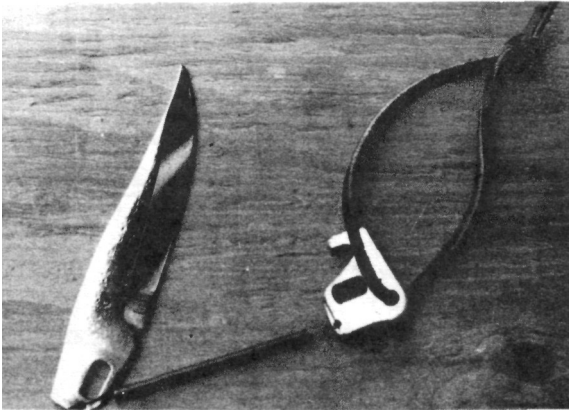
Blade and catch mechanism with operating spring of string pull design.
