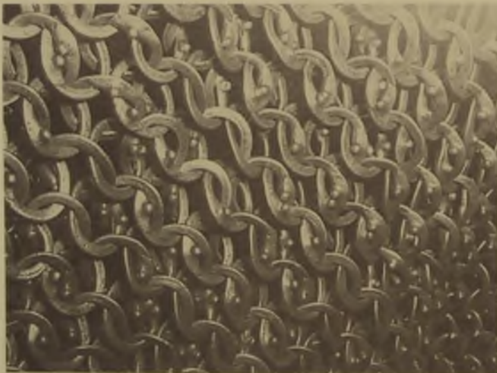
Figure 20-3. Close-up of mail from A.D. 1060. Notice the flattened wire and the rivets.
