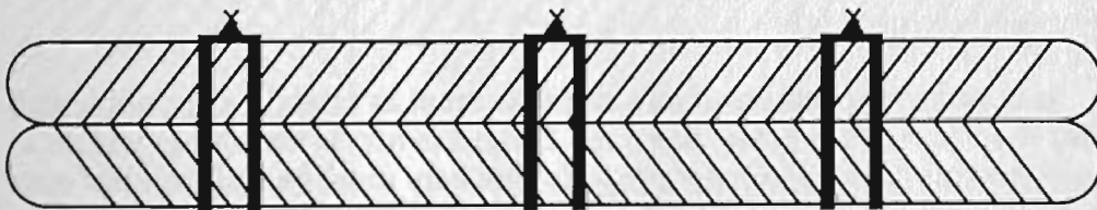
Figure 21. Bind the cores securely with heavy wire to ensure that the pieces do not shift while welding.
