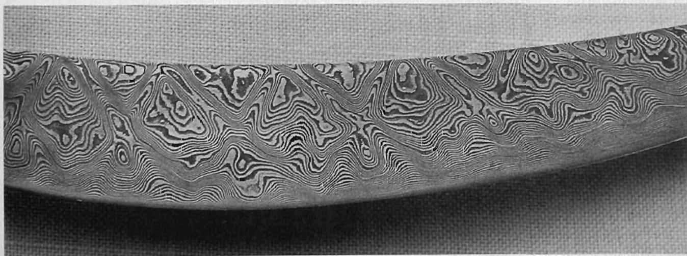
A butterfly pattern made by Wally Hayes. Materials are high-carbon and low-carbon steels. (Photo by Jim Weyer)
