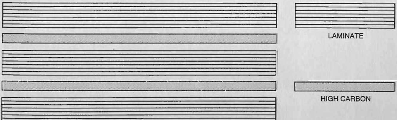
Figure 10. Material positioning for hugs and kisses pattern prior to welding.
