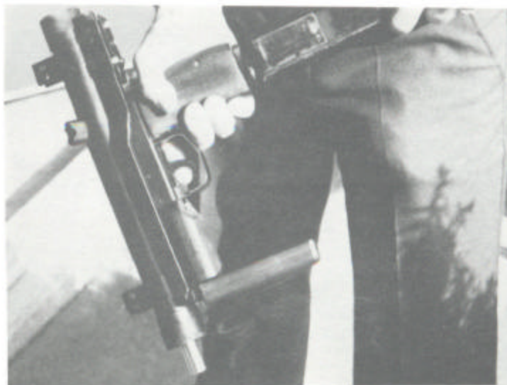
Inserting the magazine. Note the cocking handle locked in the rear position.
