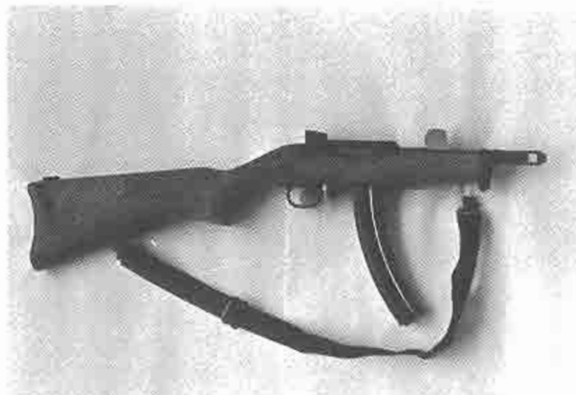
Same weapon with sling placed under the weapon unhooked from swivel attachment.
