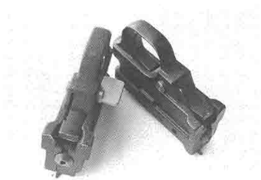
Bottom view showing the trigger housing assembly of the push-button-type safety of the factory (right) and the easily manipulated selector-lever-type of the converted model (left).
