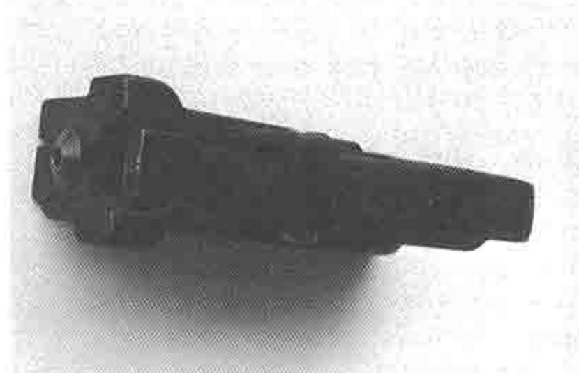
Photo shows the slave pin assembled in the selector pin hole. This pin must be in place prior to assembling the weapon to the stock. After the gun has been assembled to the stock, and the stock screw has been tightened, the slave pin is pushed out by the selector lever pin.
