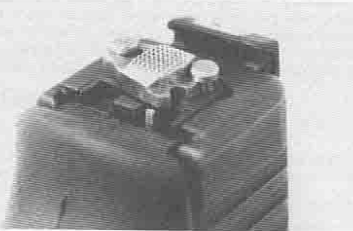
The fully assembled fire-selector mechanism seen mounted to the back of the slide cover plate.
