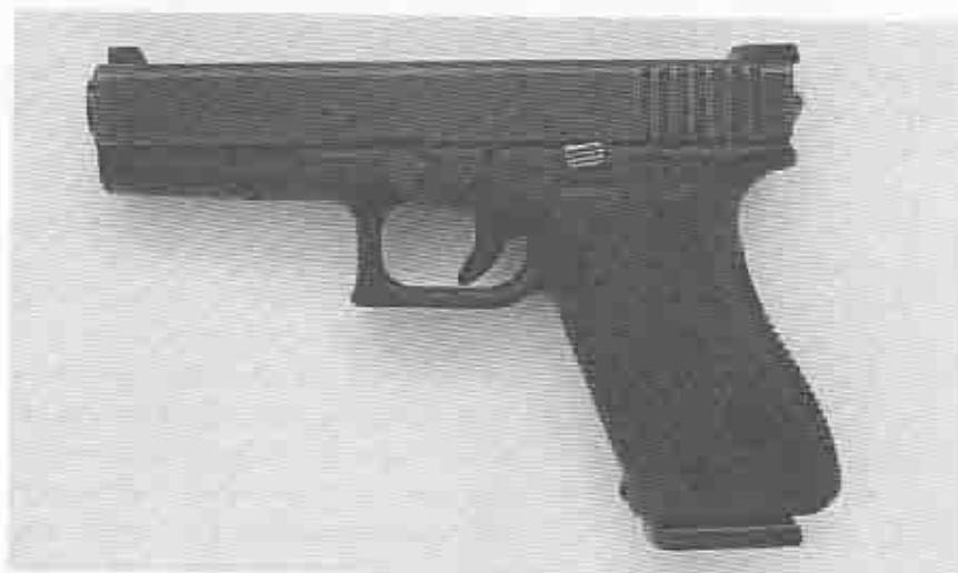
Left-side view of the newly converted Model 21. The only external difference from the original semiauto format is the fire selector mounted at the back of the slide.
