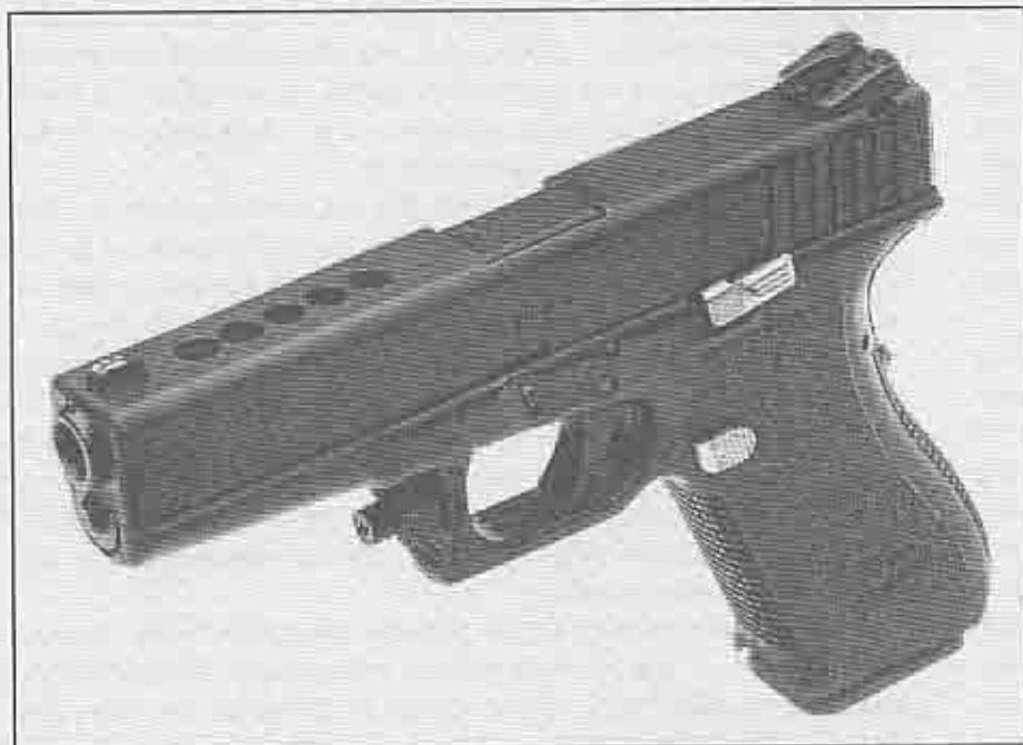
Left-side view of the magnificent Glock Model 18 machine pistol chambered for the 9mm Parabellum. The fire selector is mounted at the rear of the slide and is set for full-auto firing. This is the 21st century machine pistol. (inset) Aro-Tek's laser-equipped Law 2000. This is a highly customized Glock featuring the Hybrid compensator system complemented by the company's own custom accessories.
