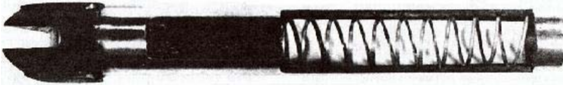
Finished Slide Assembly With Recoil Spring In Place
