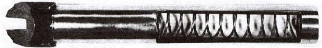
Finished Slide Assembly With Recoil Spring In Place
