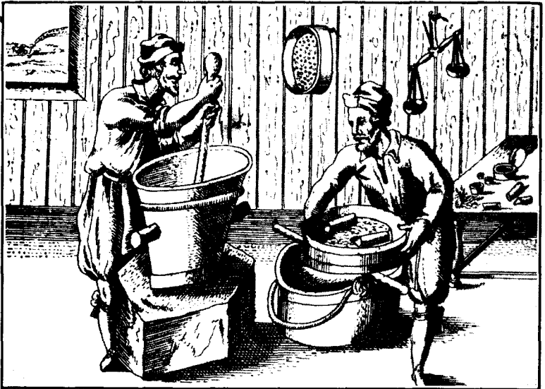
FIGURE 18. Gunpowder Manufacture, Lorraine, 1630. After the materials had been intimately ground together in the mortar, the mixture was moistened with water, or with a solution of camphor in brandy, or with other material, and formed into grains by rubbing through a sieve.
