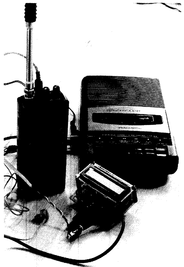
Figure 14. A homemade "Y" adapter will allow you to listen to DTMF tones while you decode them.
