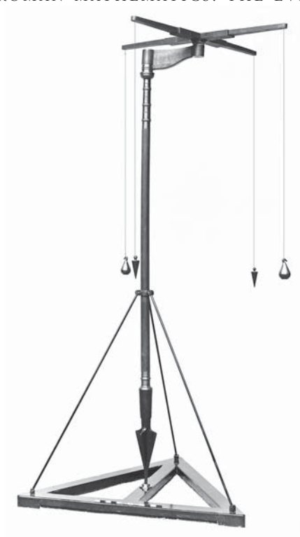
Figure 5.4 Reconstruction of a groma from Pompeii, c. first century AD (© copyright Science Museum/Science and Society Picture Library, London)
