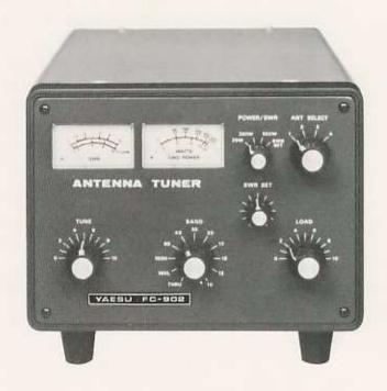
The FC-902 antenna coupler is designed for low and medium power applications in the HF amateur bands from 160 through 10 meters. It is designed to minimize the adverse effects of high SWR on a coaxial line or wire antenna which may result in difficulty in tuning a transmitter designed to work into a resistive 50 ohm load.
