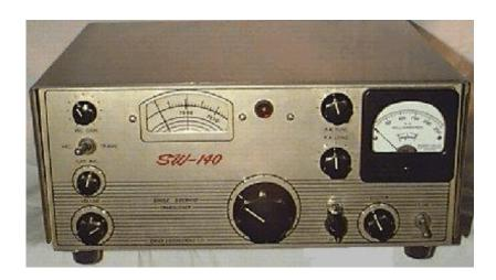
The Swan SW-140 monoband 40m HF rig shown here is one of the gold coloured units that were first produced when Herb Johnson began manufacturing amateur radios. Designed for mobile, portable or fixed station use. Introductory price, in 1962, was \$275.00 US available from your dealer. TECHNICAL SPECIFICATIONS....
