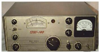
The Swan SW-140 monoband 40m HF rig shown here is one of the gold coloured units that were first produced when Herb Johnson began manufacturing amateur radios. Designed for mobile, portable or fixed station use. Introductory price, in 1962, was \$275.00 US available from your dealer.
