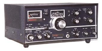
The Swan 750CW was billed as "The CW Man's Dream" in 1977. It featured 700 watts PEP output, and 400 watts DC input on CW. Some of the standard items included were CW audio filter selectable 80 or 100 Hz., CW sidetone monitor with adjustable pitch and volume control, 80 thru 10 meters USB, LSB, and CW, selectable 25 or 100 Khz crystal calibrator, and a
