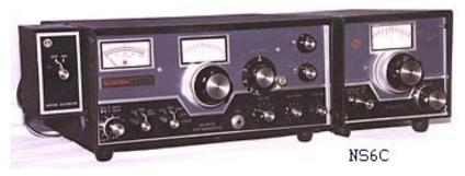
The Swan 250 is a 6 meter transceiver which was first introduced in the spring of 1965. With two 6146B tubes as the PA, this radio is rated at 240 watts PEP on SSB, 180 watts CW, and 75 watts on AM. Band coverage is 50 to 54 Mc, and the pi network coupling provides for
