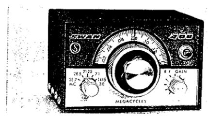
Model 406 Frequency Control Unit is designed for full phone band coverage of 80, 40, 20 and 15 me meters, plus two 200 ke segments of the 10-meter band. The unit is specifically intended for mobile operation, and provisions for mobile mounting have been incorporated.
