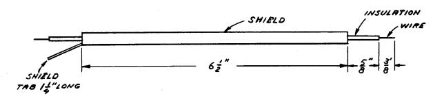
A. Replace shielded lead from L4 to grid of second converter, V3 with above lead, placing it under phasing control shaft as shown in the pictorial diagram below.
