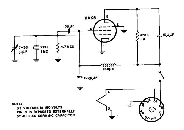
XCU-109 Crystal Calibrator Schematic Diagram
