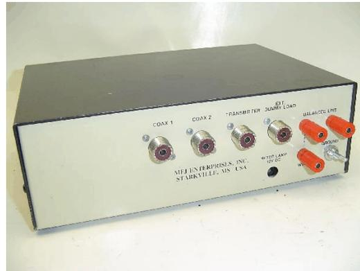
**MFJ MODEL 948 ANTENNA TUNER - HANDLES UP TO 300 WATTS OF RF - COVERS 160 THRU 10 METERS - BUILT IN 4:1 BALUN FOR MATCHING OPEN WIRE FEEDERS - COMBINATION POWER/SWR METER - PERFECT FOR MATCHING ALL TYPES OF ANTENNA**
