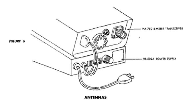
The HA-750 is designed to be used with any 6-meter antenna providing 30-100 ohms (Nominal 50 ohms) impedance. Antenna polarization is very important at these frequencies and should be considered when choosing an antenna. Generally speaking, the antenna polarization should be compatible with that of the stations you will normally be in contact with.
