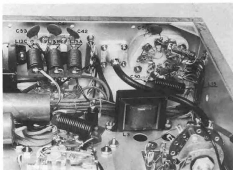
Figure 10d—Line Filter, VFO Socket Wiring Detail
