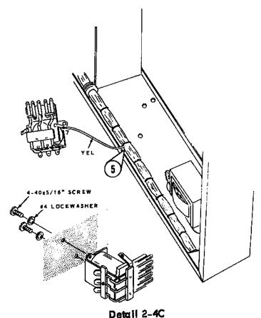
Connect the wires from BO#5 of the cable assembly to the relay as follows:
