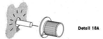
the AF Gain control knob setscrew should be tightened against the flat of the shaft.
