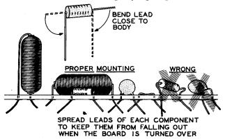
NOTE: Exercise care not to damage resistors or capacitors when bending the leads as shown.
