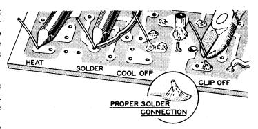
to be soldered, as shown. The iron should be held so that solder is not likely to flow to adjacent foil conductors or connections. The solder should immediately be placed between the iron and the joint to be soldered. Remove the length of solder as soon as its end begins to melt and flow onto the lead and foil. Hold the tip of the iron in place only until the solder begins to flow outward over the foil; then remove the iron quickly.
