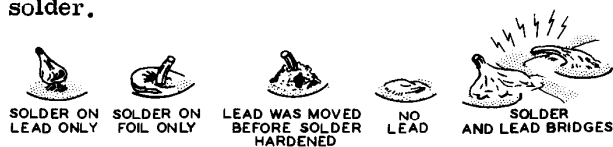
IMPROPER SOLDER CONNECTIONS
