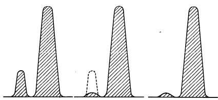
With Selective Switch in XTAL Sharp position identify the weaker amplitude—Tune Receiver to the weaker.
