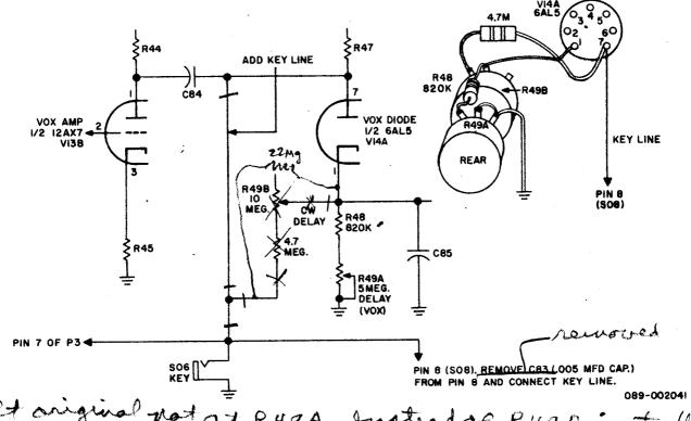
Left original pot at R49A. Instead of R49B installed PROCEDURE: a 22 meg resistar (2 sec sud delay).
