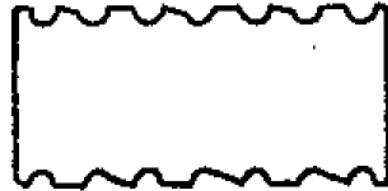
SSB SIGNAL, TONE INPUT AUDIO DISTORTION EXCESSIVE AUDIO INPUT EXCESSIVE DISTORTION IN AUDIO OSCILLATOR
