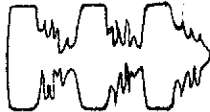
SSB SIGNAL, VOICE INPUT. SQUARING AUDIO PEAKS. EXCESSIVE SPEECH GAIN
