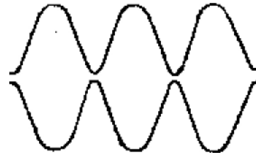
DOUBLE SIDEBAND AM WITH CARRIER 100% MODULATED
