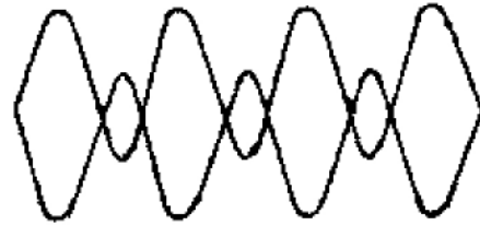
DSB DOUBLE SIDEBAND REDUCED CARRIER OBTAINED BY REDUCING CARRIER LEVEL AND INCREASING AUDIO INPUT LEVEL.
