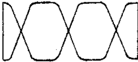
SSB WITH CARRIER, TONE INPUT. 1. EXCESSIVE AUDIO SIGNAL 2. INSUFFICIENT ANT. LOADING
