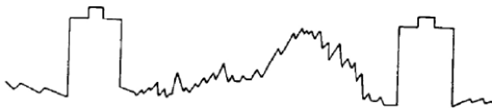
Figure 4—Normal Video and Sync Signal.
