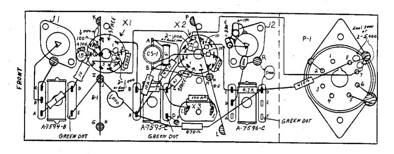
Fig. 1. Parts layout of CB-6 converter for 7 to 11 Mc. output as viewed from underside of chassis. For other outputs, see changes listed in section on "Selecting the Output IF Frequency".
