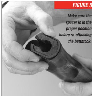
shooters, install this spacer with the R facing out, toward the end of the buttstock, so its thicker side is on the left side of the receiver. This casts the stock slightly to the right, away from the face of a right-handed shooter. Turn the spacer around so the L is facing out and it will cast the stock to the left.
