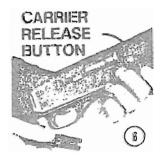
in the "on safe" position close the action with the carrier release button. With the carrier
