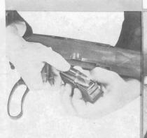
Load magazine with four cartridges.
