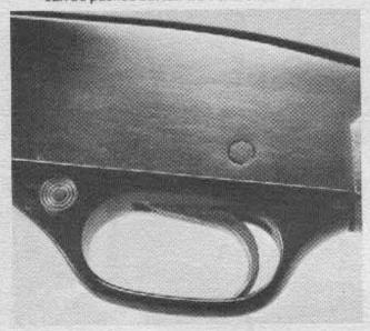
Tip the trigger housing down at the rear, and move it slightly toward the rear to disengage its forward stud from its recess inside the receiver. Remove the trigger group downward.
