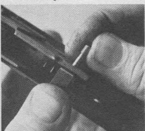
16. Remove the sear/disconnector assembly upward. The sear and its spring are a permanent assembly inside the disconnector, the pivot pin being riveted in place at the factory. Routine removal is unwise in normal disassembly.
