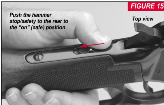
94. It serves to drop an internal hammer block that is positioned between the hammer and receiver. The hammer block prevents the hammer from striking the firing pin until you pull the trigger to fire the rifle.
