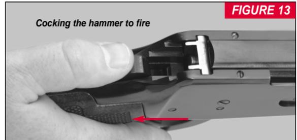
With a loaded cartridge in the chamber, the manual hammer stop/safety in the "on" position, the hammer in the safety (rebound) position and your finger off the trigger:
