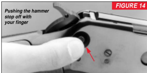
2. Place the manual hammer stop in the “off” position (See Figure 14) by pushing it from right to left.
