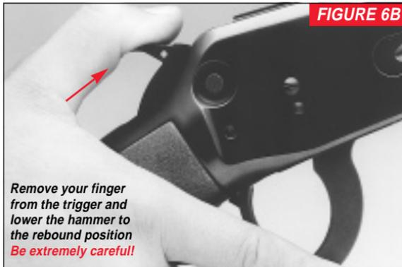
3. While holding the hammer back apply just enough pressure on the trigger and finger lever to release the hammer from the full-cock position. Immediately remove your finger from the trigger and slowly and carefully allow the hammer to lower into the rebound position (See Figure 6-B).
