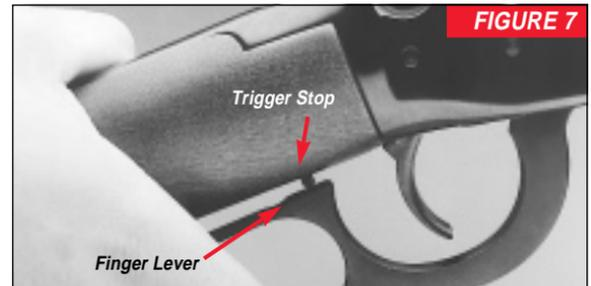
on this rifle is engaged, it is designed to prevent accidental discharge. However, this mechanism will not necessarily prevent the accidental discharge of this firearm as a result of jarring or abuse such as occurs when a firearm is dropped.
