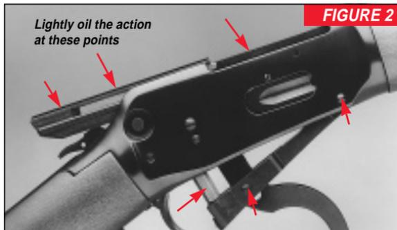
the inside of the barrel, receiver, cartridge feed mechanism and the action/chamber areas. A high quality, light gun oil should be used to remove this compound and to give your new gun its first lubrication. Clean the barrel using a cleaning rod and patch as explained under “Cleaning and Maintenance Suggestions” found later in this manual. First lubrication suggestions are outlined below.
