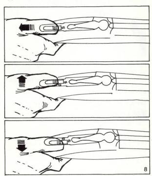
A mechanical switchover in the selective trigger system gives you second-shot reliability because recoil is not required to activate the second shot. In case of misfire because of a defective shell, pull the trigger again—the second barrel will fire.
