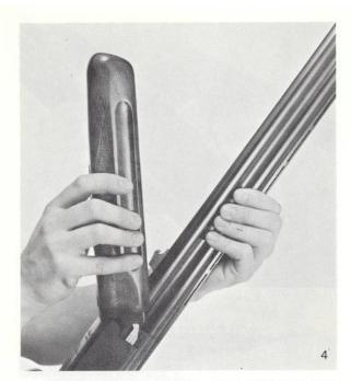
To attach the forearm to the barrels, hold the gun at the barrels with the butt of the stock resting on your thigh with the trigger guard up. Engage the rear of the forearm at the front of the receiver and pivot it into place, then snap the forearm release closed. (Fig. 4)
