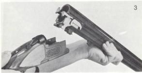
To attach the barrels to the receiver, grasp the receiver at the pistol grip and tuck the butt section between your body and arm just above the waist. Grasp the barrels with the other hand above the forearm lug. (Fig. 3) Hook the barrel lug recess (A) over the hinge-pin (G, Fig. 2) in the front of the receiver, and pivot the rear of the barrels into the receiver by lifting sharply on the barrels.
