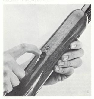
First, remove the forearm by pulling the forearm release latch located on the underside of the forearm and pivot the front of the forearm away from the barrels. (Fig. 1) If the gun is dry, put one or two drops of gun oil on (A) lug recess of the forward barrel lug, (B-C) all sides of both barrel lugs, and at (D,E,F) end of forearm bracket. (Fig. 2)
